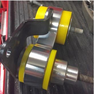
7. Using a torque wrench tighten bolts No:5,6,7 & 8 to 48nm/34 lb-ft.
