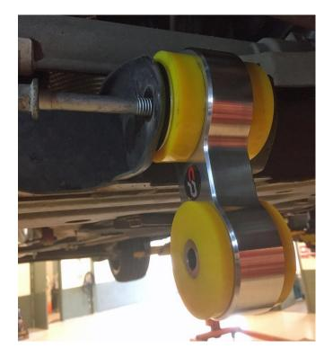
6. Install the remaining 3 x 13mm gearbox bolts (no 5,6 & 8) and support bracket – please ensure the correct sequence is used of bolt, support bracket, thick washer, torque mount and then spacer and pictured below
