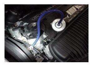
5) Remove small plastic shroud above cam cover between cam pulleys and oil filler cap, cut vacuum pipe, fit plastic tee piece and silicone hose, attach dump valve to silicone hose.
