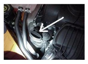
3) Push canister out of mounting bracket in the direction of the arrow, then remove bracket.
