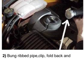
secure with tie wrap on strut brace.
