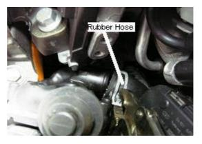
6) Remove this rubber hose and reverse it. Use the 2nd jubilee clip on the other end. If you do not reverse this hose the dump valve will rest on the engine.
