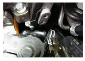
4) Pull canister to one side while clamping the spring clip on the inlet hose then remove the canister and spring clip.
