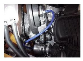
**7)** Fit dump valve into inlet hose using 3rd Jubilee clip to secure.
