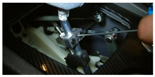
7. Relocate cable into carrier extension – ensure it is located securely
