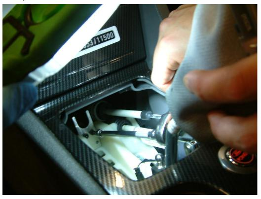
5. Install ball joint relocation bracket onto gear lever rod tighten using 4mm Allen key
