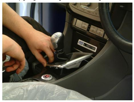
2. Prise cable from lever ball joint using large screw driver
