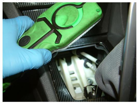
4. Install into position cable carrier extension – tighten using 4mm Allen key
