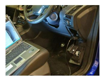
**2.3** Press the ignition start button to bring on the dash warning lights – DO NOT START THE ENGINE
