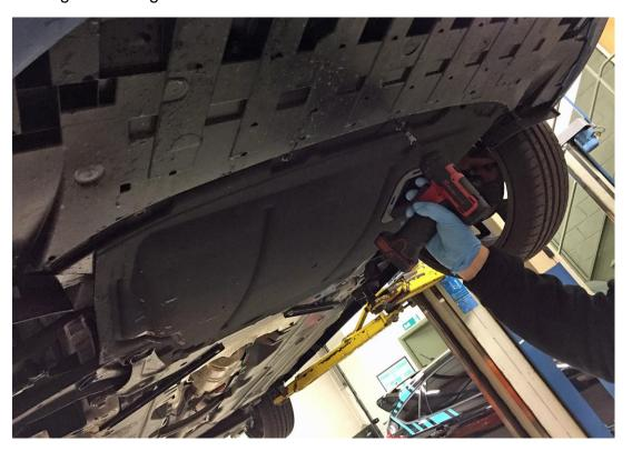
3. Remove the 1 x 16mm Bolt & 1 x 15mm Bolt retaining the existing mount (retain parts for reinstall later)
