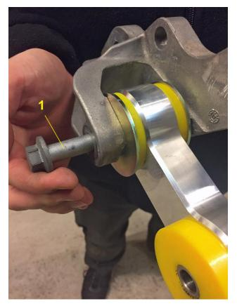
7. Locate the mount and alloy spacer onto the subframe and install the 15mm bolt No2 <u>finger tight only</u>
