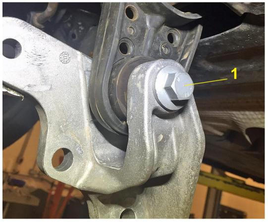
6. Locate the CP Mount and 2 x 2.5 x 60mm washers into the OE mount bracket as pictured and install the 15mm bolt No 1 finger tight only
