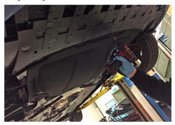
3. Using a 15mm spanner loosen the 15mm bolt No1
