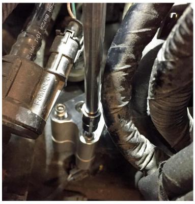
9. Reinstall the cable connector onto the quick shift ball joint as shown below (6)
