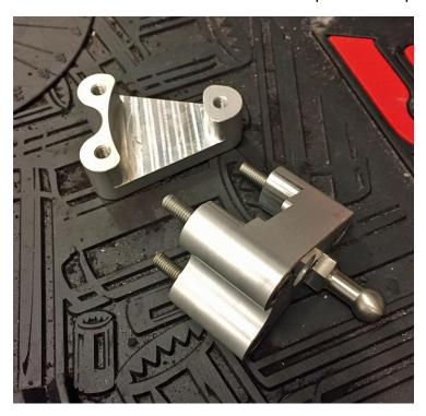
7. Locate both halves of quick shift around the selector arm as pictured and finger tighten the 3 x M5 bolts (use a small drop of thread lock on each bolt)
