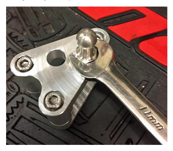
6. Remove the 3 x M5 bolts and separate the quick shift
