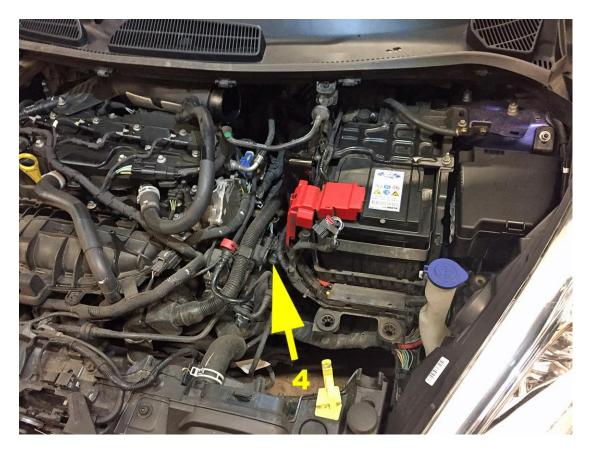
4. Using either a trim tool or large flat bladed screw driver prise the cable connector upwards away from the gear box arm (5)
