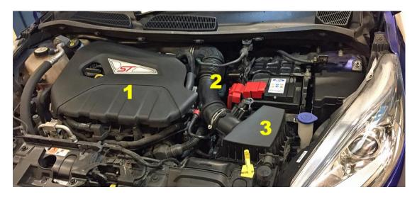
12. Take care to connect the vacuum pipe to the induction pipe and the MAF sensor to the airbox
