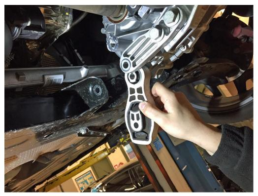
5. On the smaller end of the CP Mount protrude the bush just far enough to be locate the 1.4mm spacer washer - see photo below
