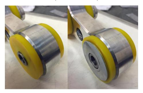
6. Install the CP Mount onto the subframe and loosely install the 15mm bolt
