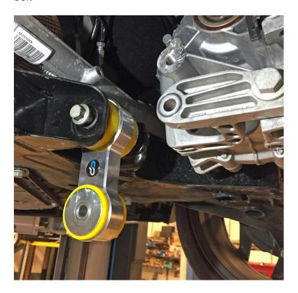
7. Swing the mount into the engine bracket ensuring the correct location of the spacer washer and loosely install the 16mm bolt
