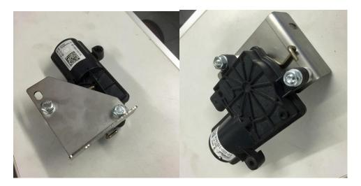
6. Locate the bracket/valve assembly onto the car using the M10 bolts/washers and nuts supplied – see image below
