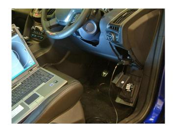
**3.2** Switch on the ignition either by pressing the start button or turning the key to bring on the dash warning lights – DO NOT START THE ENGINE
