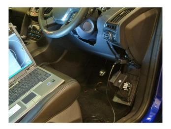
**2.3** Press the ignition start button to bring on the dash warning lights – DO NOT START THE ENGINE
